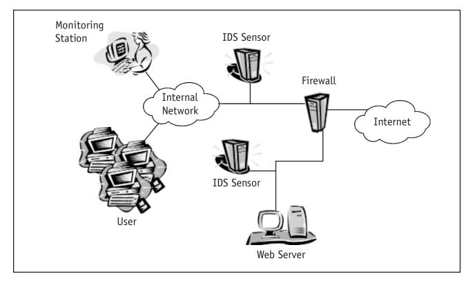
Figure 3. This diagram shows placement of a traditional network based IDS with two sensors on separate network segments that communicate with a monitoring station on the internal network.
