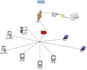
Fig2. Network Based Intrusion Detection System
