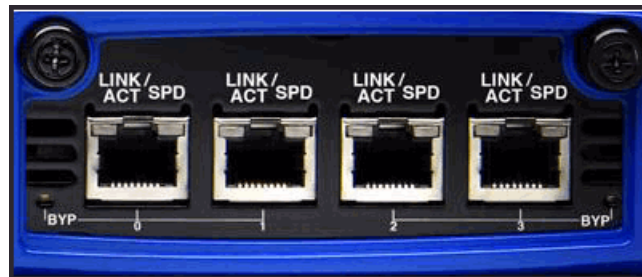
Figure 4: Copper Port LEDs
