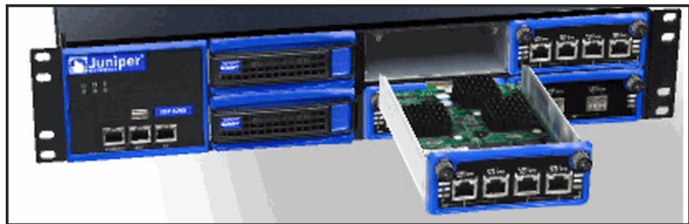
Figure 25: Replacing a Blank Tray with an I/O Module Tray
