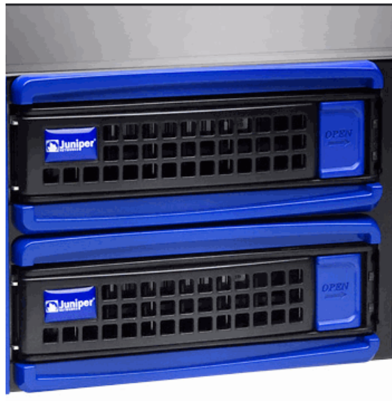
Figure 26: Hard Drive Latch in Closed Position
