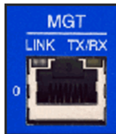
Figure 2: Management Interface Port LEDs
