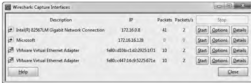
Figure 3-4: Selecting an interface on which to perform your packet capture
